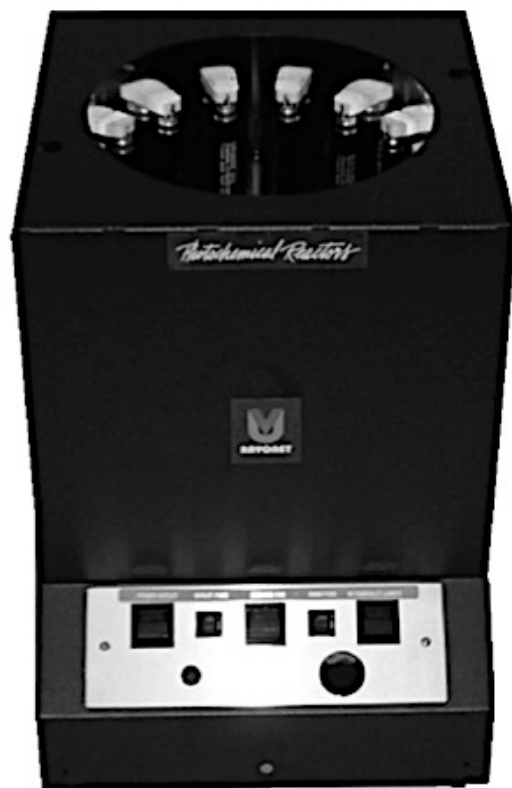
Figure 3.10 Rayonet photochemical reactor ( external configuration ). Reproduced by permission of Southern New England Ultra Violet Company
