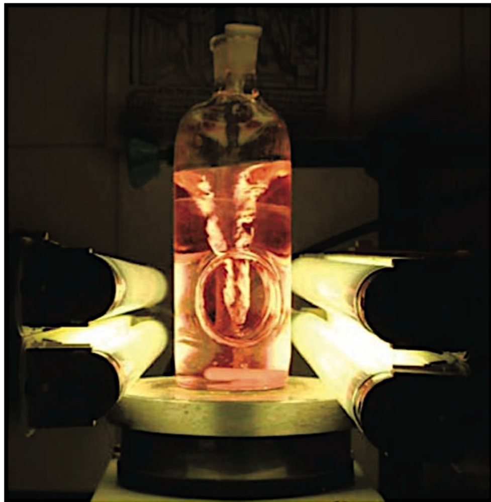
Figure 1.3 Two pairs of lamps used for external irradiation. In the arrangement shown, only a small fraction of the light flux is used.
